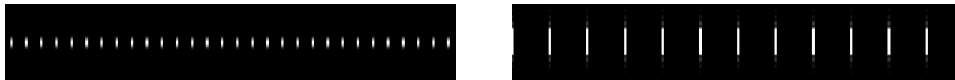
Figure 10: Grating structure with a multiple-period size. The Fourier transform is sharp and background-free.
