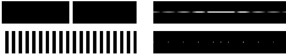
Figure 20: Slit width equates one half of the period: The minima of the slit diffraction function (top right) correspond to the maxima N = \pm 2, \pm 4, \dots of the grating diffraction resulting in missing maxima (bottom right).
