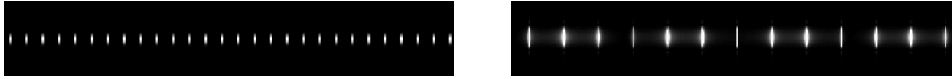
Figure 11: Grating structure with a size not equal to a multiple of the period (left), and corresponding Fourier transform (right).
