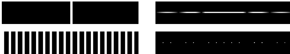
Figure 21: Slit width equates one third of the period: The minima of the slit diffraction function (top right) correspond to the maxima N = \pm 3, \pm 6, \dots (result bottom right).
