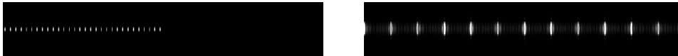
Figure 12: Zero padding: Grating structure of Fig. 10 padded with a zero matrix of the same size. In the Fourier transform the minor structures of the pattern are now visible.
